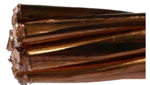
Common scissors: remember to use a file in order to remove the copper in excess. Make sure to follow the stranding direction.
