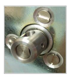
Reassembly the motor assy back, don't forget the keyway, put momentary bolts and check the rotator, if runs OK, remove the bolts, seal the motor cover against the rotator main body using polyuretane sealant or similar glue, screw down the bolts and clean the sealant that come out from the flanges. Make sure that the sealant fully cover the flanges border.
